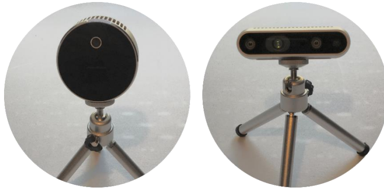
Figure 2-9. MEMS LiDAR cameras (left) and stereoscopic depth cameras (right)
