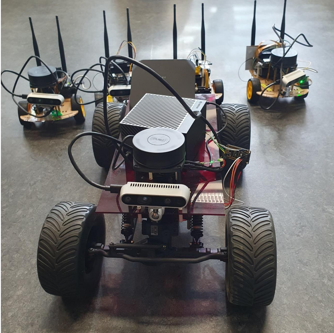
Figure 4-23. Ground vehicle robots equip with sensors.
