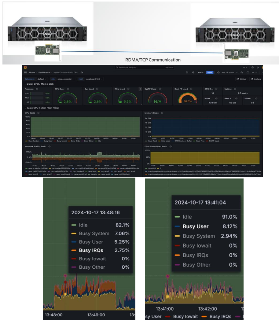
Figure 3-23: (top) testbed setup for RDMA assessment. (middle) Graphana view of RDMA performance. (lower left) Performance using traditional TCP data transfer. (lower right) performance using RDMA.
